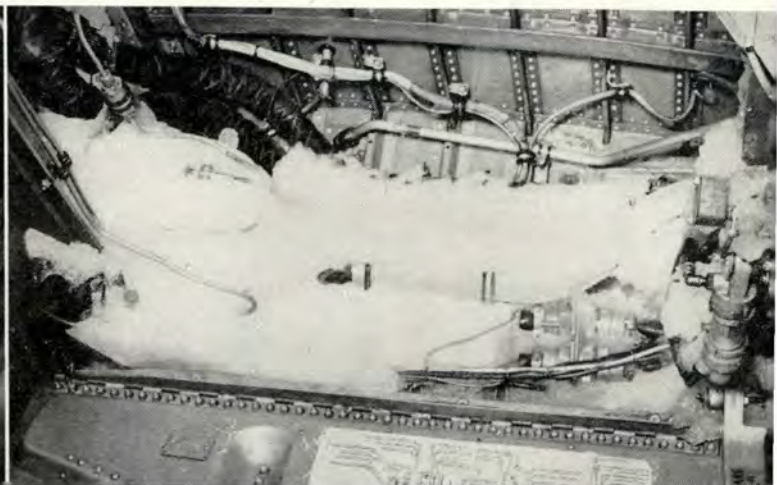
When you take off from a slush covered runway, here is the result.
